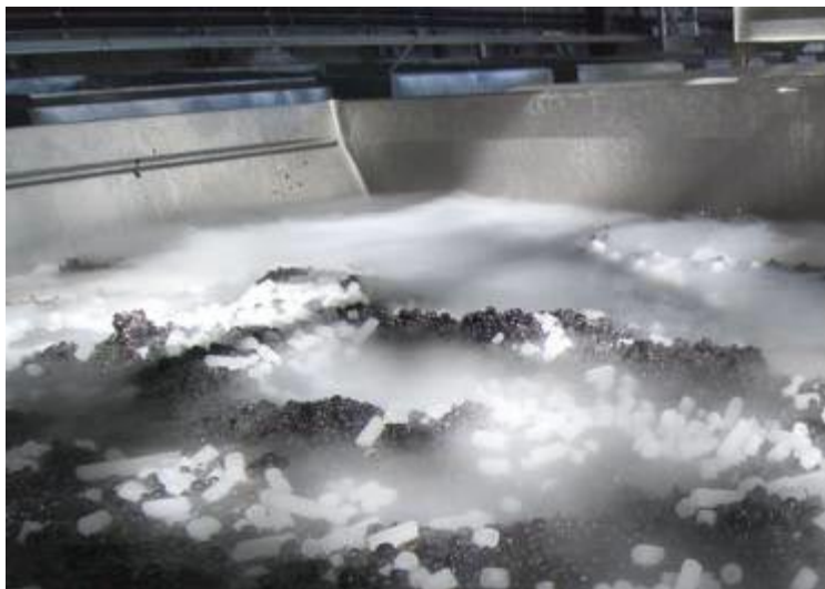
Dry ice layered in a fermenter to protect grapes during cold soak.
